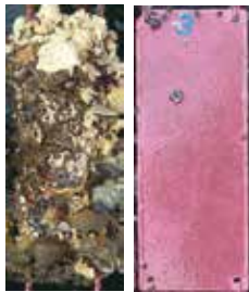
Left: Steel plate WITHOUT antifouling Right: Steel plate WITH antifouling
