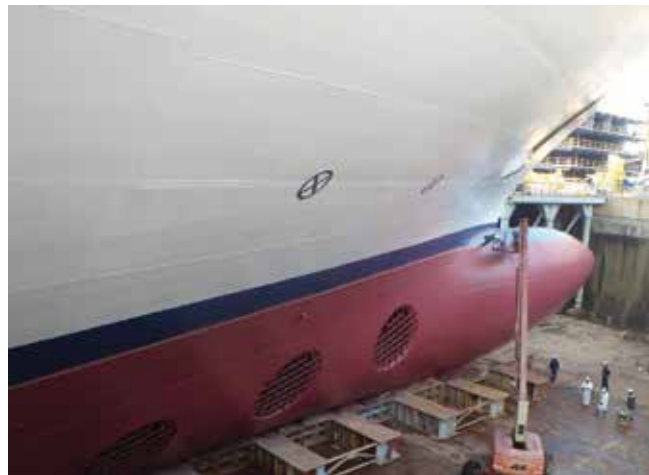
Application of antifouling coating (large vessel)
