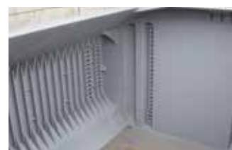
Abrasion resistance coating for Cargo Hold
